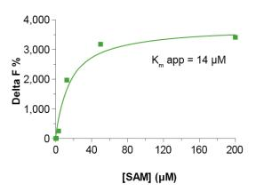
This step enables the determination of Km for SAM. The Km value was determined with 40 ng/well EZH2(Y641) complex and 400 nM biotinylated H3(1-50)me0 substrate in the enzymatic step. We recommend testing SAM concentrations ranging from 200  $\mu$ M to 0.195  $\mu$ M (serial dilutions). The enzyme reaction was stopped at the optimal incubation period (RT, 180 min) by adding the detection reagents. The 14  $\mu$ M Km value for SAM was determined from this experiment using a Michaelis-Menten plot.
